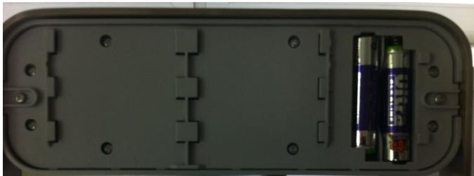
Place 2 AAA batteries in the position indicated in the battery compartment. When finished, slide the panel back into place.
