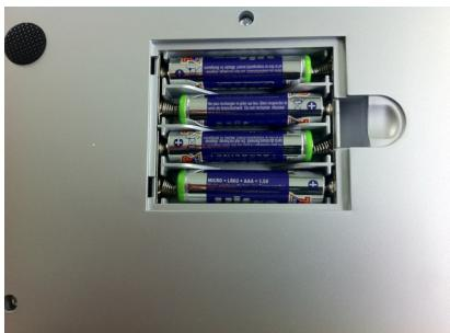
Place 4x AAA batteries in the position indicated in the battery compartment. When finished, put the battery panel back in place.
