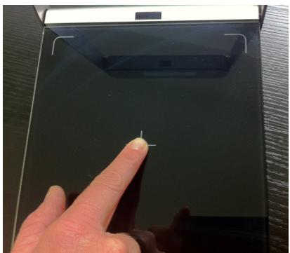
If left in the ready position for more than approx. 3 minutes and 30 seconds, the scale will automatically shut off to conserve battery life. To turn the device back on while in the ready position, press approx. 2 seconds on the weighing platform until the signal tone sounds and the display lights up.
