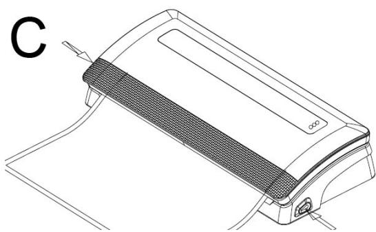
5. The vacuum packaging is done (LED 11). Press the Release button (2) (image C) to open the cover and take out the packed bags.
