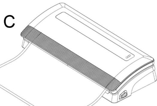
3. Close the upper lid and hold it down tightly on both side of the machine by two hands till you hear motor working and keep it for a few seconds (image C) . The machine will then suck the cover down tightly and seal this bag, and automatically stop when the bag is sealed.
