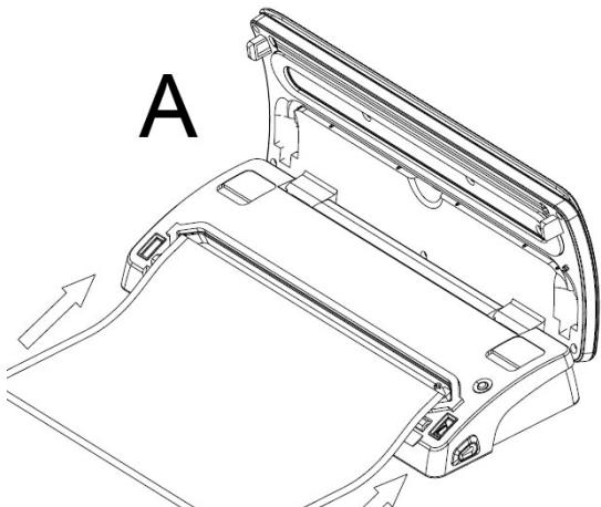
3. Place the open end of the bag as seen on the image (A) within the vacuum chamber are. Make sure the air intake (3) is not covered by the bag, otherwise the vacuum can not be generated correctly.
