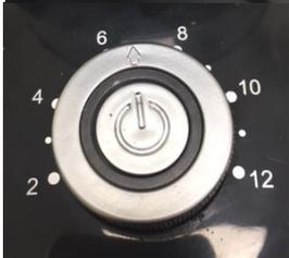
9. Turn the knob for duration of grinding to set to the desired amount of cups
