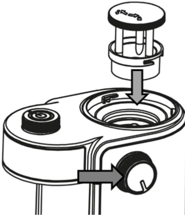
Place the grinder and then turn it slightly back and forth so that the grinder will slide down into the guidance.
