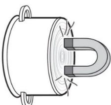
Ensure that the pot bears an inscription stating its suitability for cooking with induction current, or perform the following magnet test:
