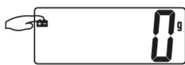
When the display indicates low battery
