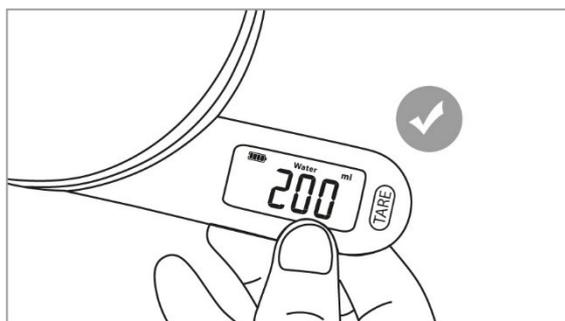
Press the UNIT button (at backside of display) to interchange the unit between g, oz, Water ml, Milk ml. Select the UNIT button before weighing. The TARE button cannot be pressed at the same time as the UNIT button.
