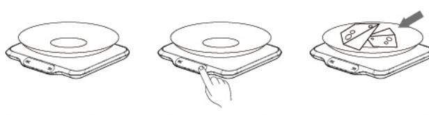
**TARE** Place an empty container on the scale. The LED display will now show the weight of the container.
