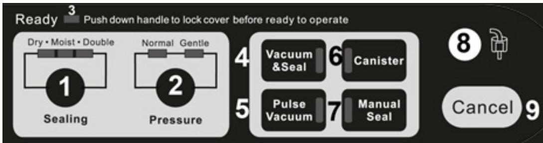
**1 Sealing time (Sealing):** Three buttons for choosing the best bag seal time
