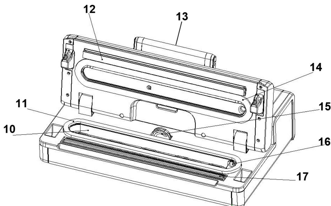
**10 Vacuum chamber:** Position the open end of the bag inside the chamber.
