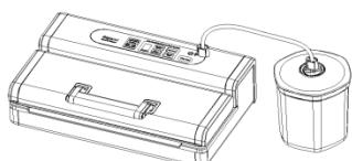
Insert one end of the hose into the hose port and another end of the hose into the center hole of the canister cover.
