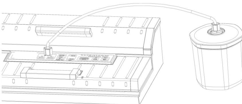
Insert one end of the hose into the air intake and another end of the hose into the center hole of the canister cover.
