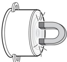
◆ Place a magnet (e.g. a magnet from a magnetic board) close to the base of your cooking pot. If it is strongly attracted then you can use the cooking pot on the induction cooktop.
