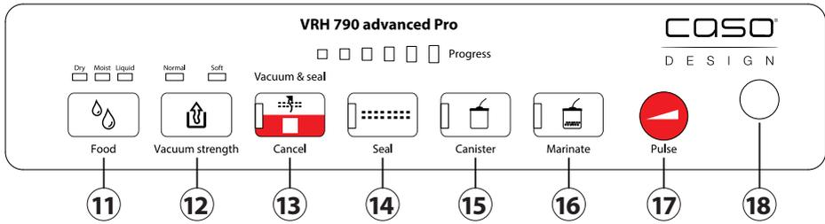
Progress – LED light indicates progress of the relevant process.
