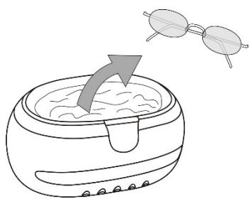
The unit will stop automatically after 3 minutes. If another cleaning is needed, press the ON button again.
