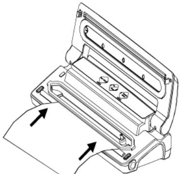
1. Unroll the bag to the desired length and cut the bag to the appropriate length with precise and clear cut.
