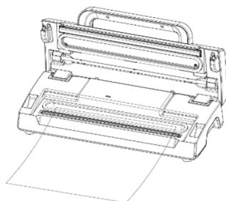
Clean and straighten the open end of the bag--ensure there are no wrinkles or ripples.
