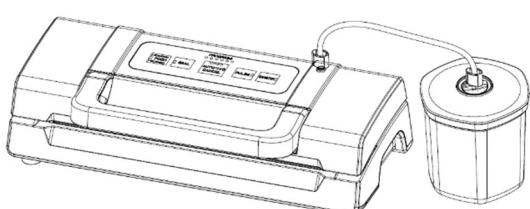
Insert one end of the hose into the hose port and another end of the hose into the center hole of the canister cover.
