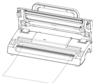
Put one end of the bag on top of the sealing bar.
