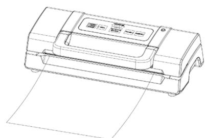
Close the lid and press the handle down firmly until the first progress LED lights up.
