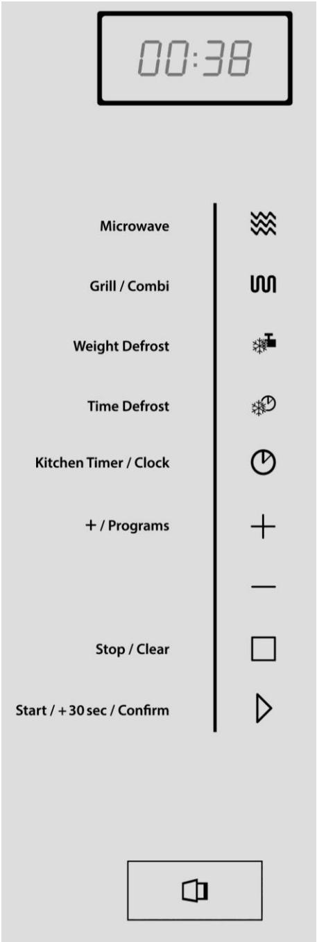
**Display panel:** Cooking time, output, function display and actual time are displayed.
