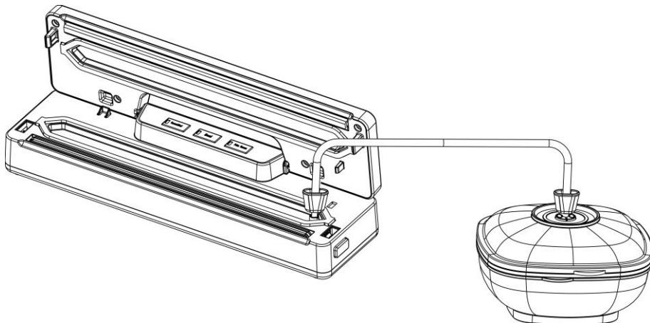
Close the lid. Attach one end of the hose at the air intake at the device and another end to the connector at canister lid or with the adapter at canister lid.
