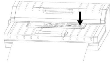
Lift the front handle to open the cover and take the bag out of the machine. The bag is then done and is ready for vacuum sealing .
