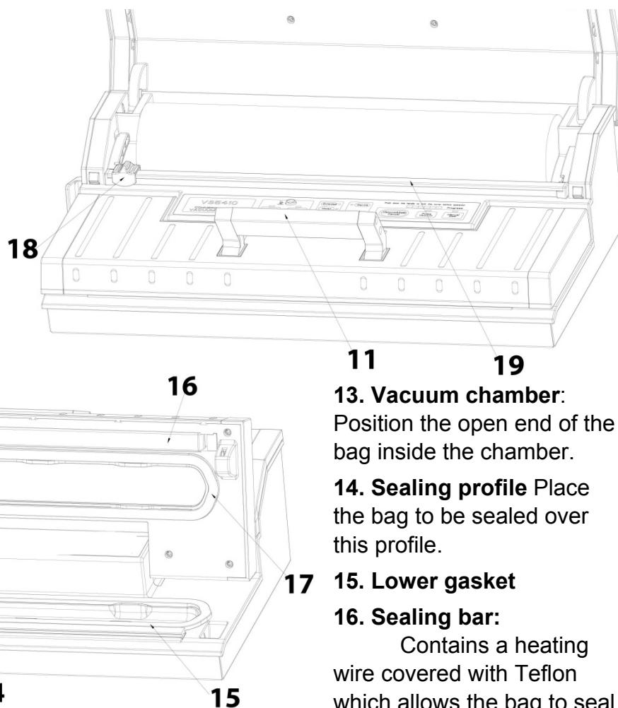
but not to stick to the strip. Place the bag to be sealed over this sealing element.
