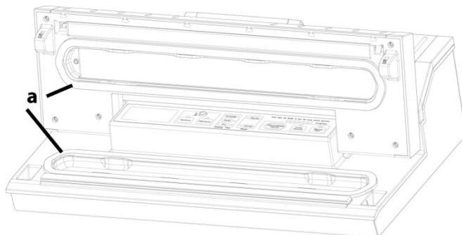
Turn off the device using the main switch. Let the device cool down completely. Open lid of the device. Take the upper/lower gasket out of the trough in the cover of device/from the trough around vacuum chamber. Insert the new gasket and push it with your fingers into the trough.
