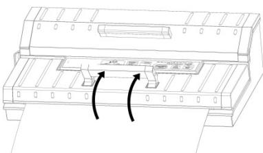
Press “Schweißen” (seal) button to start sealing the bags.
