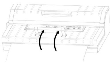
Press the “Vakuum & Schweißen” Button. The Vacuum Indicator Light, then the Sealing Indicator Light with light as the bag is automatically vacuumed and sealed. Once it is finished, both lights will turn off.
